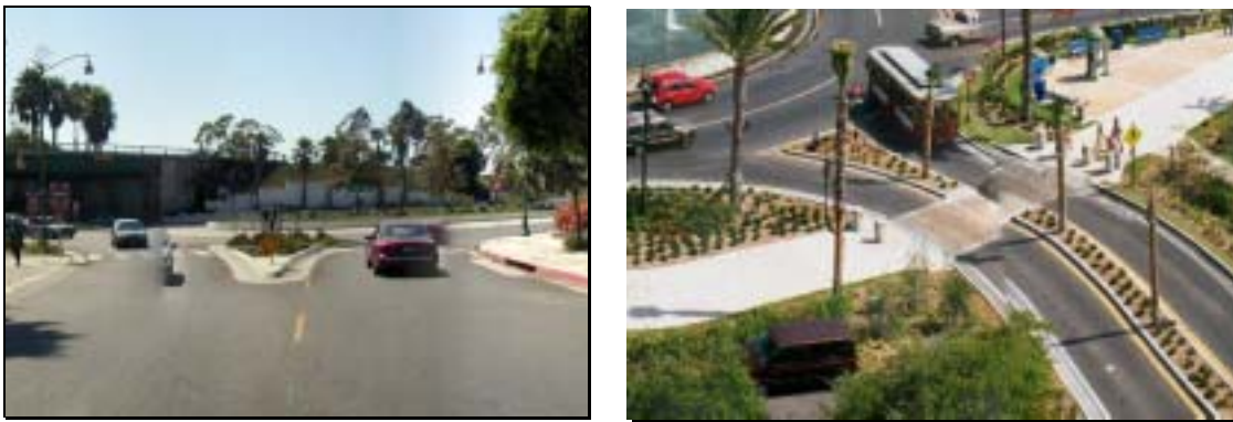
Figure 50 Median splitter islands and set-back crosswalks create safe pedestrian crossings
