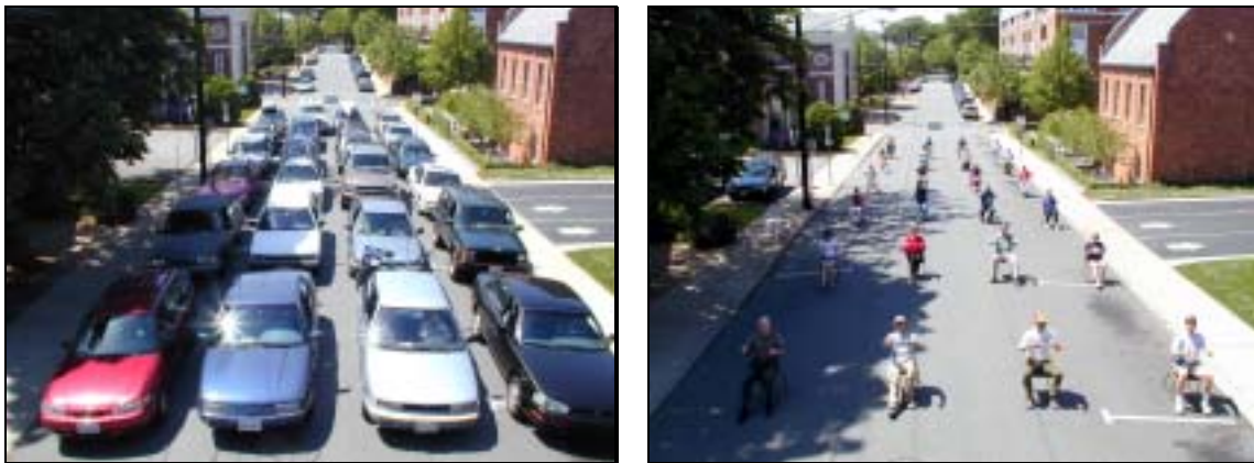
Figure 26 Many streets and highways are at capacity, can't fit more cars, and can't be widened. If we think in terms of moving people, not cars, existing streets have plenty of room for more.
