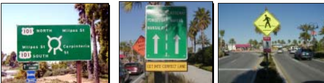
Figure 51 Signage and lane markings help drivers and pedestrians navigate a roundabout
