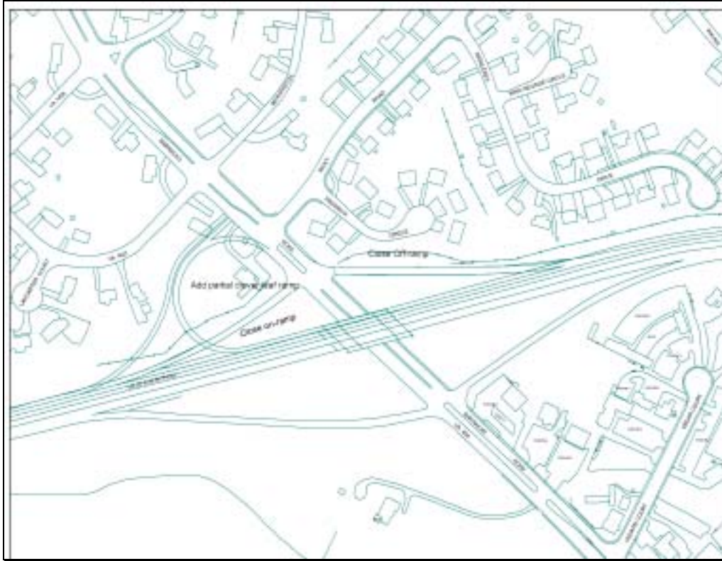
Figure 29 This option shows Barracks Road Cloverleaf with existing ramps closed and moved
