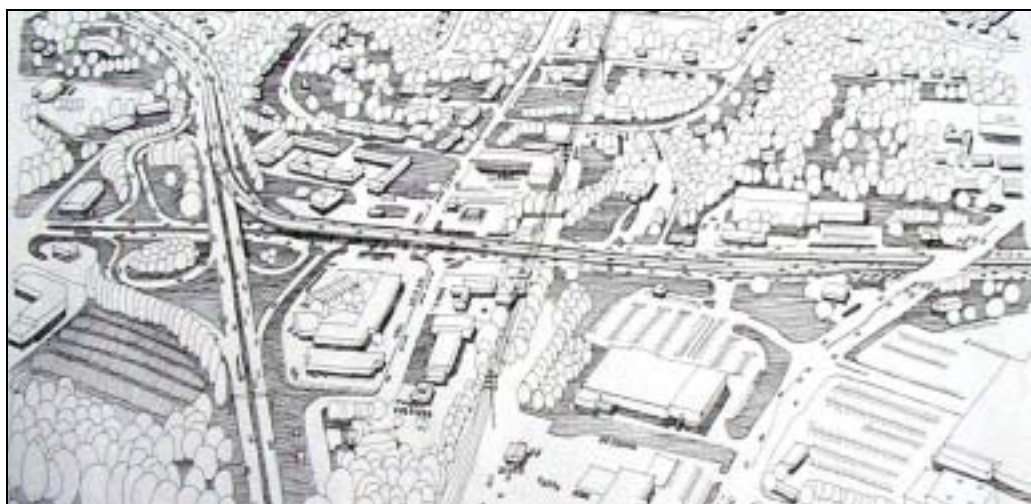
Figure 9 The Passonneau Study proposed grade separations and a flyover from 29 to the 250 Bypass
