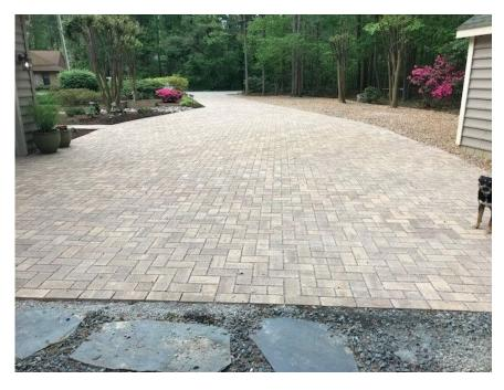
Permeable pavements replace traditional concrete or asphalt with a porous surface and underlying stone to allow for drainage. Instead of quickly moving water over the surface, permeable pavements allow water to pass through the material and percolate into the ground below. Common types of permeable pavement include pervious grid pavers, porous asphalt or concrete, and permeable interlocking pavers. These pavements offer attractive
